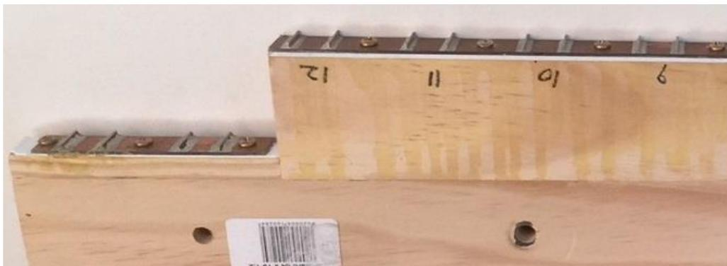
The jig bolts to the module end and gives an accurate position for any available entry/exit track.
